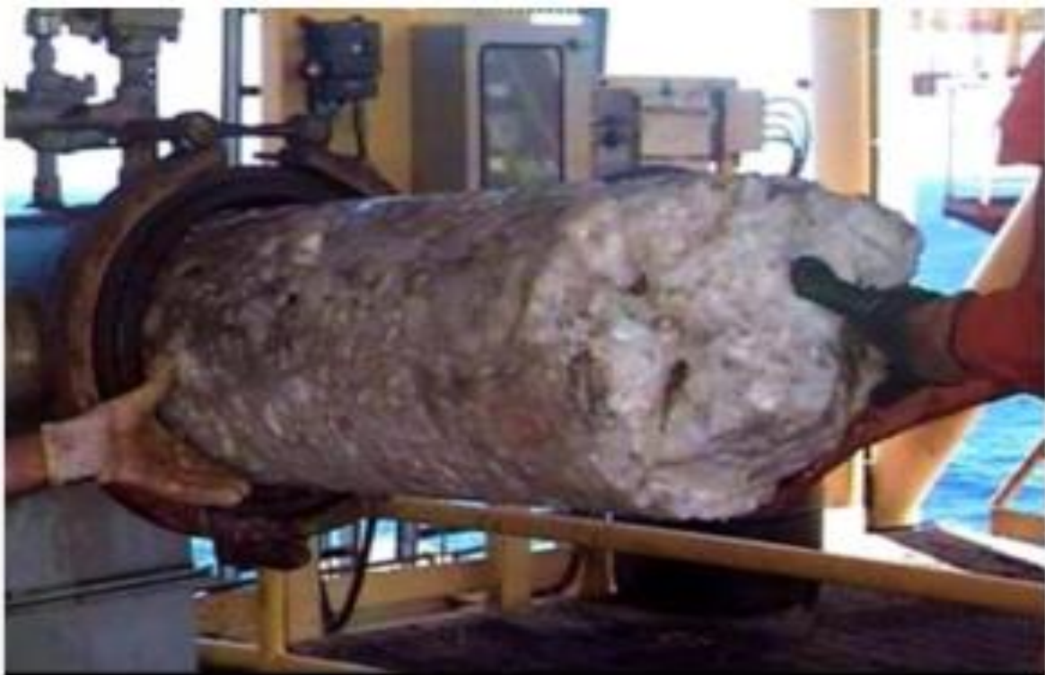
Figure 4: Hydrate formation in natural gas transmission pipeline (Fang et al., 2020).
