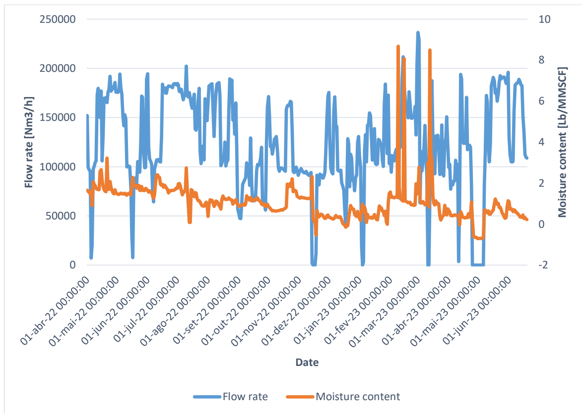
Figure 15: The effect of gas flow rate in the absorber on the moisture content in the pant.
