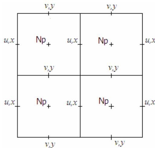
**Figure 6:** Model meshgrid
