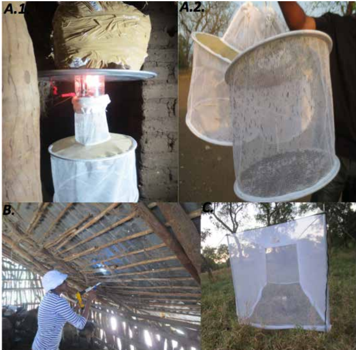
Figure 11. Host-seeking adult mosquito collections using light trap (A.1. and A.2.), animal shelter (B.), and Tent/Net trap (C). Both "A" and "C" were baited with attractant CO 2 .
