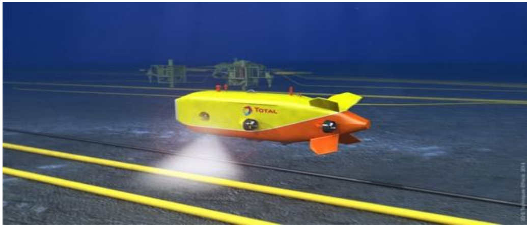
Figure 27. ROV - Last and high technology from Total for monitor subsea facilities (pipes) for flow assurance.
