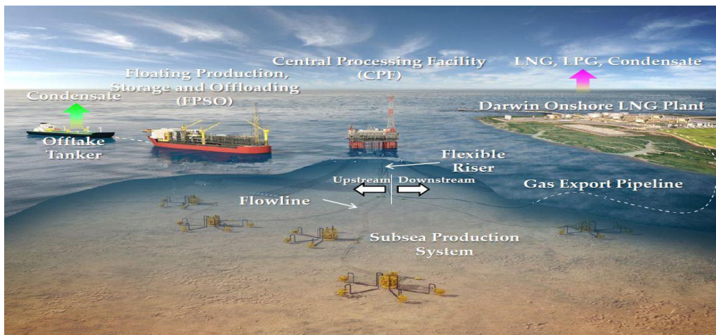
Figure 24. Generalised facilities in offshore (upstream) and onshore environment for gas production.
