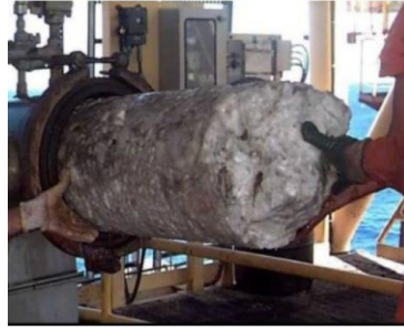
Figure 9. Hydrate Plug Formed in a Subsea Hydrocarbon.
