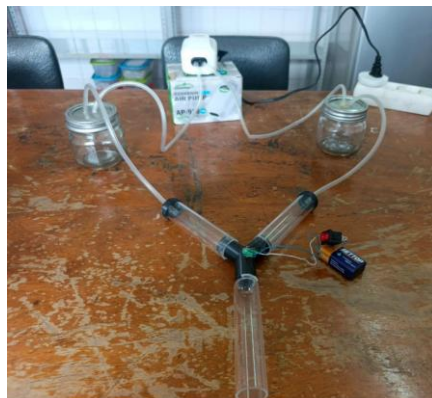
Figure 11. Assembled Y tube olfactometer with odors sources, air pump and tubes.
